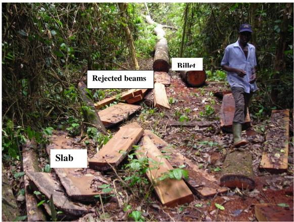
Figure 13.3: Types of solid wood residue generated during chainsaw milling process. Picture from Nkrabia FR showing residue from a sawn mahogany tree
