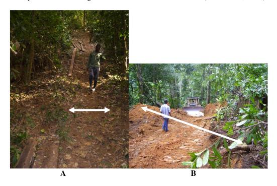
Figure 13.2: Pictures showing the widths of - (A) foot path used by CSM operators to cart lumber from stump site at Tano Offin FR and (B) Primary trail used by skidding machines to move logs from stump site to loading bay at Asenayo FR.
