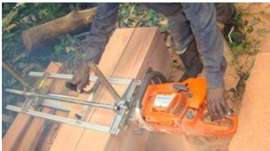
Plate 4: Milling with a frame attachment
